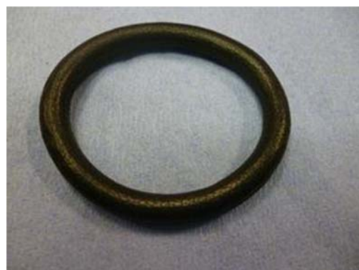
Figure 1: Standard EPDM after 24 hours 316°C in steam. Specimen is warped with surface cracking.
