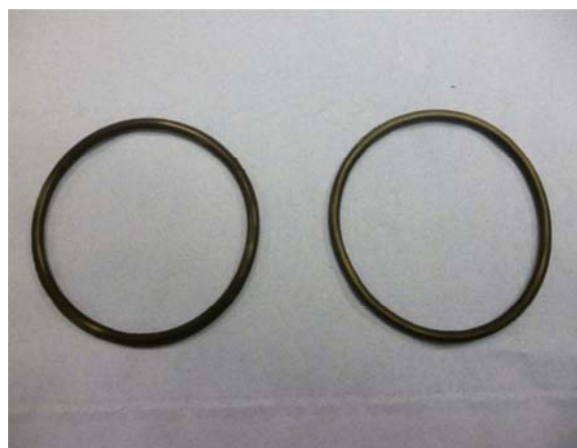
Figure 5: Left is an unaged sample, right is a steam aged specimen at 288°C for 168 hours.
