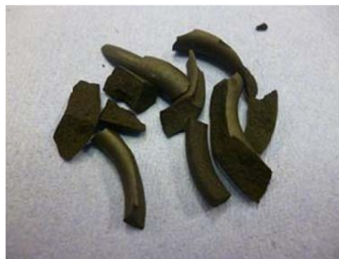
Figure 3: FKM Copolymer after 24 hours in 316°C steam.
