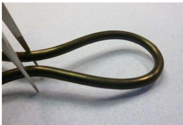
Figure 6: EnDura E90SR remains flexible without cracking in steam at 316°C for 24 hours.
