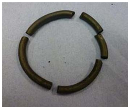
Figure 2: FKM Terpolymer after 24 hours in 316°C steam.
